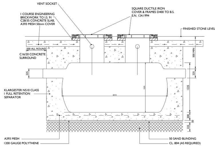
**SECTION THROUGH CLASS I FULL RETENTION SEPARATOR**
