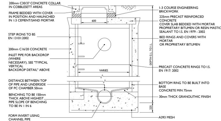
**PRECAST RING MANHOLE - SECTION**
