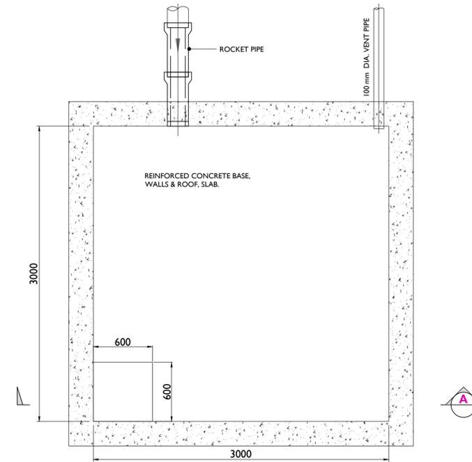
**STANDARD FOUL WATER HOLDING TANK - ELEVATION**
