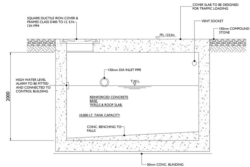
**STANDARD FOUL WATER HOLDING TANK - SECTION A-A**
