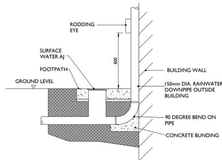
**RAINWATER DOWNPIPE DETAIL**
